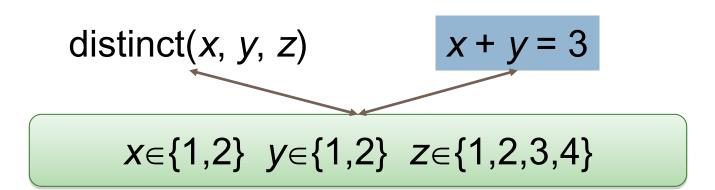
Strengthen store by constraint propagation
