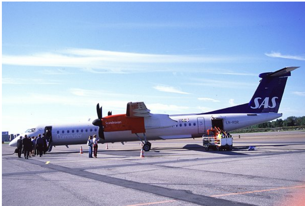
Figure 2.1: An SAS aircraft at work. This is the De Havilland Canada Dash 8 Q400, commonly known as the “Q400”. The Q400 is normally flown with two air hostesses. It has two engines of 5000hp each, composite 6 bladed propellers, a cruise speed of 670km/h, and takes around 70 passengers. Thanks to Hans Norman/www.scanliners.com for the picture. Please visit http://www.scanliners.com/ for pictures of the other aircraft in the SAS fleet!
