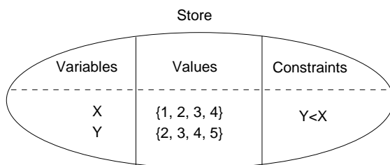
Figure 1.1: An abstract representation of a store with its variables, values and constraints.
